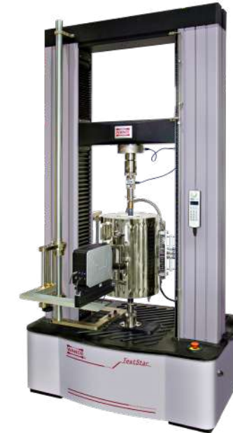
TSE-D with furnace and video extensometer
