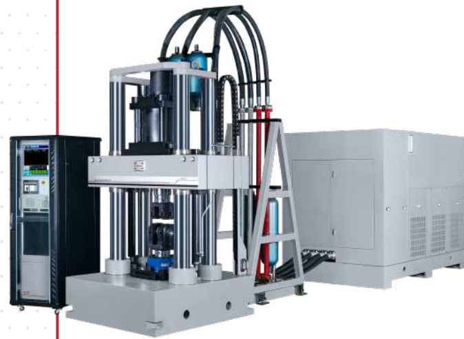
▲ Engine connecting rod fatigue test (800kN)
