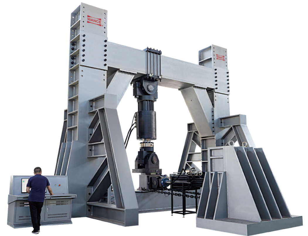
▲ Multi-channel coordinated loading test system
