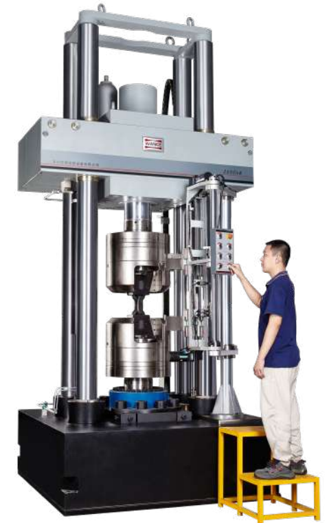
▲ 2500kN servo-hydraulic fatigue testing machine
