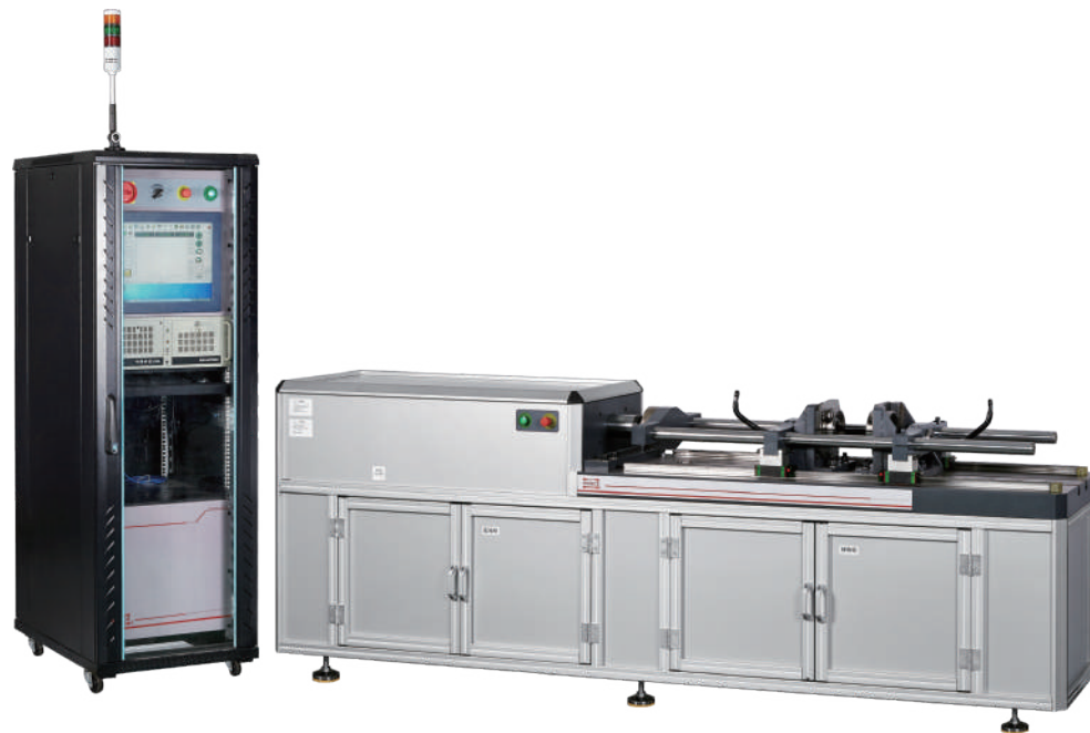
▲ Automobile stabilizer bar fatigue testing machine
