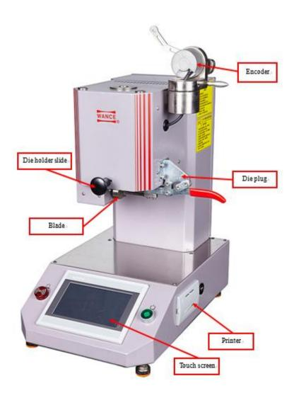
The main body of the equipment is made of 1.5mm thick high-quality alloy, equipped with 7-inch color display. The operation interface can be switched between Chinese and English, and the friendly interface can display the test parameters in real time.
