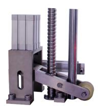
the driving cylinder is extended to prevent the sample from being subjected to secondary impact.
