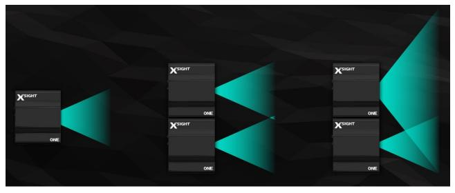
In cases when the field of view of one camera is less than 210 mm, it is not mechanically possible to merge the fields of view. That means the JOINED mode is not applicable.
